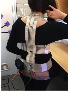
Fig. 2: StraightenUp: end result of brace with sensors, and controller box
